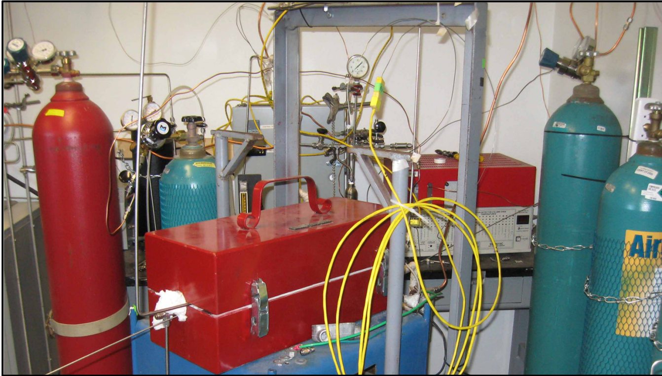
WRI flue gas membrane testing rig (flat sheet & HF modules)
